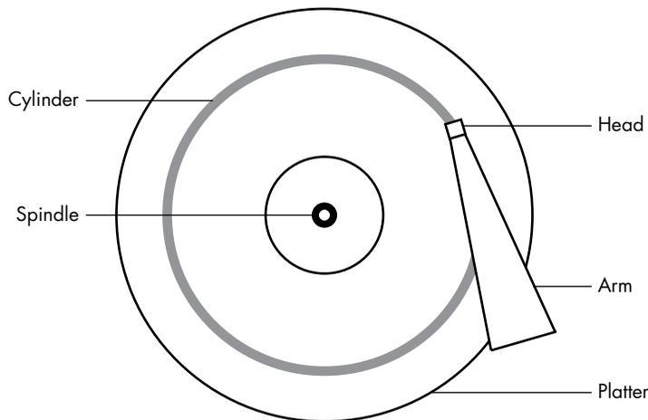
Figure 4-3: Top-down view of a hard disk
