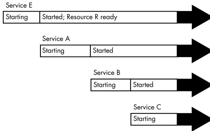
Figure 6-2: Sequential boot timeline with a resource dependency
