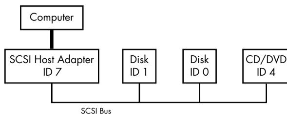
Figure 3-1: SCSI bus with host adapter and devices
