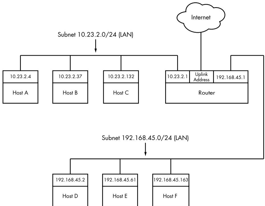
Figure 9-5: Two subnets joined with a router
