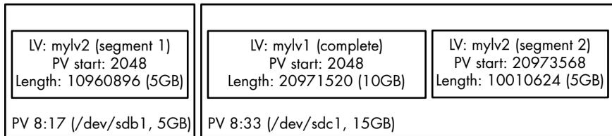
Figure 4-7: How LVM arranges `mylv1` and `mylv2`
