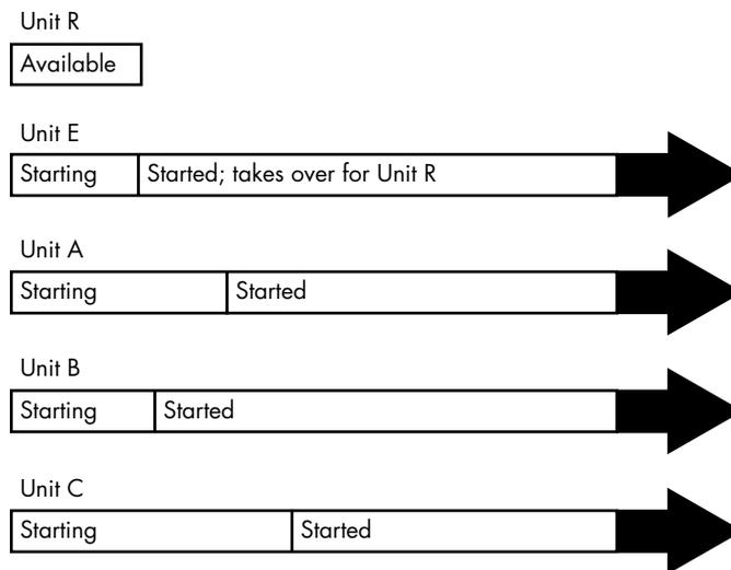
Figure 6-3: systemd boot timeline with a resource unit
