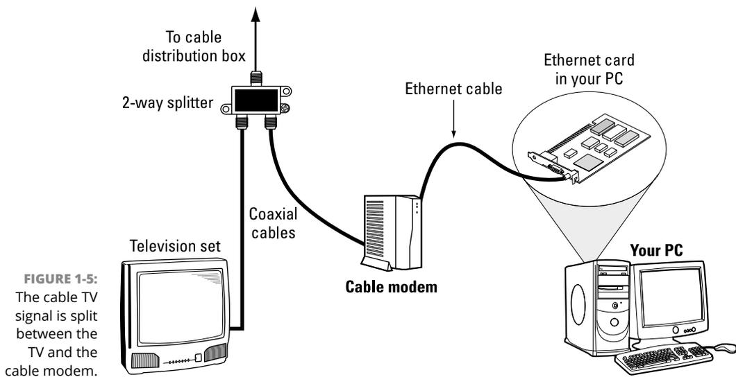
**FIGURE 1-5:** The cable TV signal is split between the TV and the cable modem.
