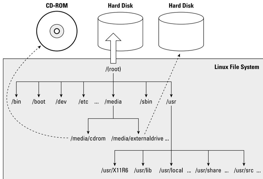
**FIGURE 4-1:** The Linux file system provides a unified view of storage that may span multiple storage devices.
