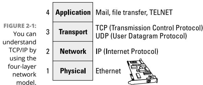
In this four-layer model, information always moves from one layer to the next. When an application sends data to another application, for example, the data goes through the layers in this order: application ↔ transport ↔ network ↔ physical. At the receiving end, the data goes up from physical ↔ network ↔ transport ↔ application.
