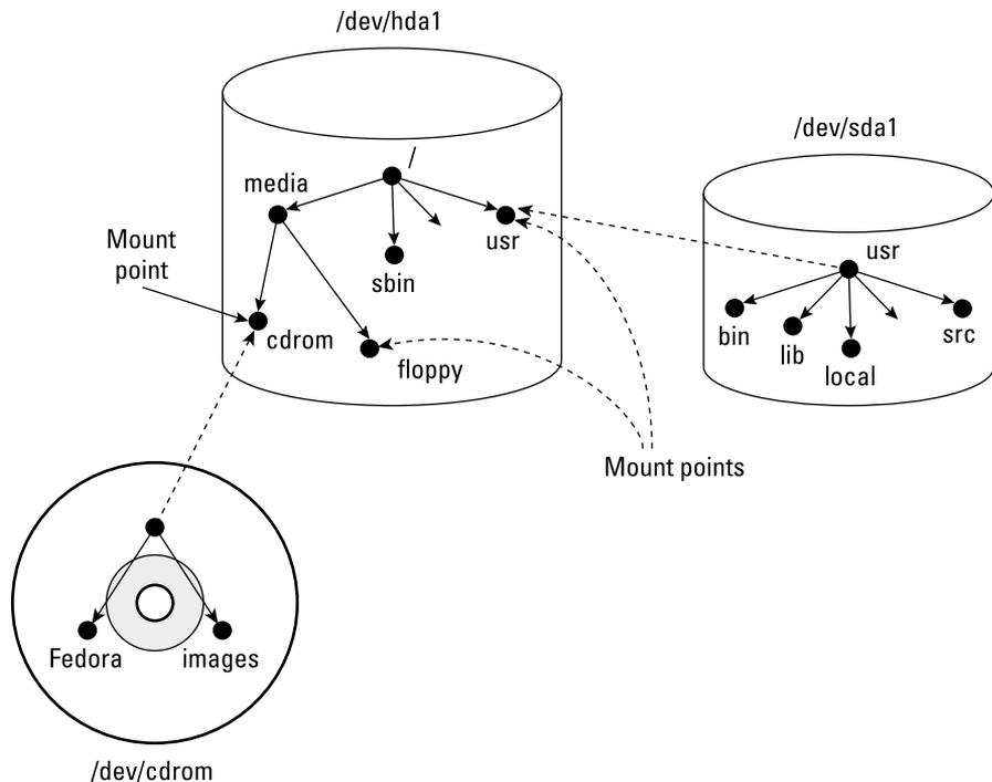
**FIGURE 3-3:** You have to mount a device on the Linux file system before accessing it.
