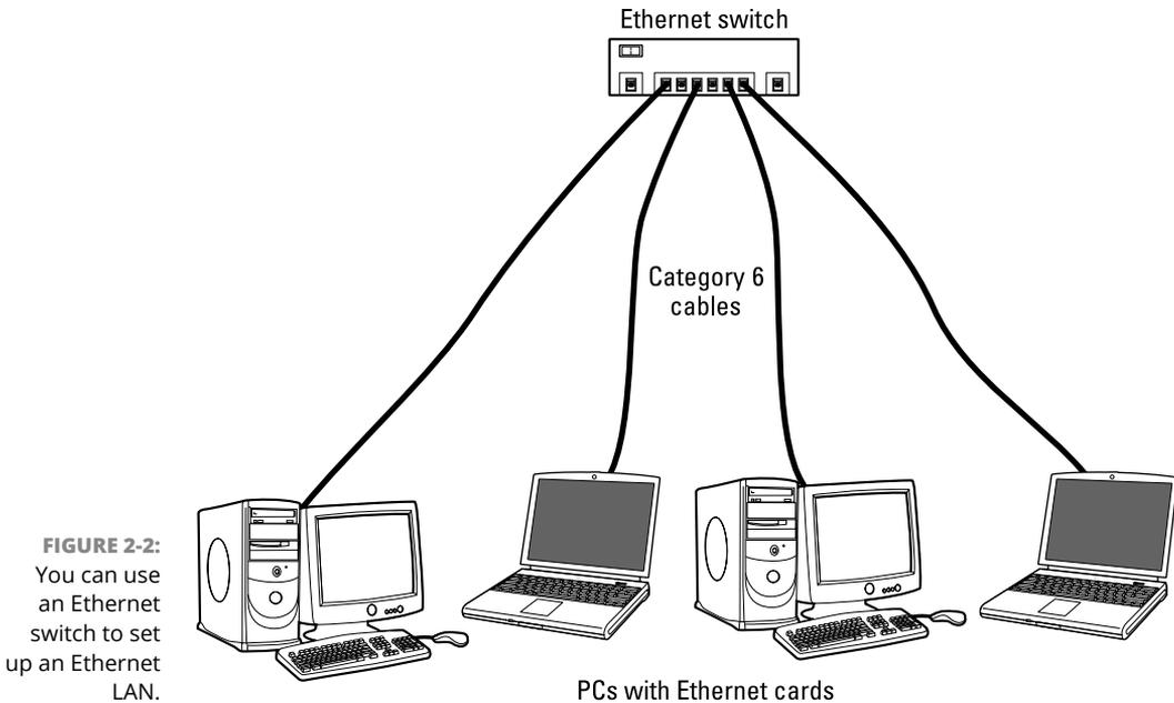
**FIGURE 2-2:** You can use an Ethernet switch to set up an Ethernet LAN.
